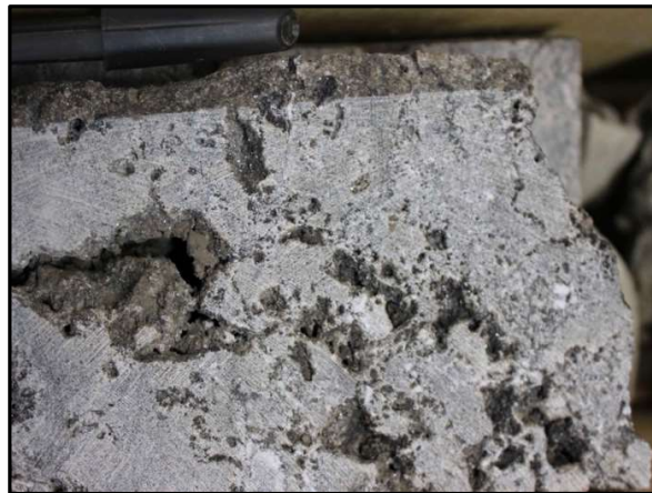
Figure 7-9: Core from 14-14-077-25 W5M with 12% porosity and 30,000 mD permeability.
